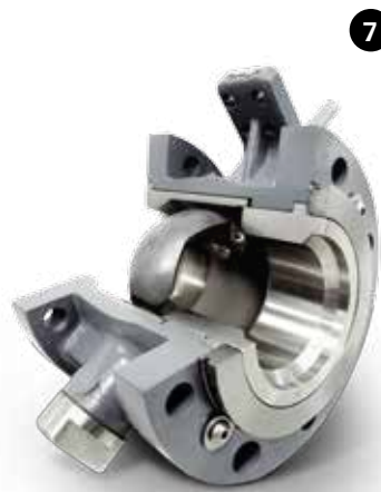
V150S erosion-resistant trim components protect the body from erosive wear and are retained without the use of press fits or threads for easy replacement.
