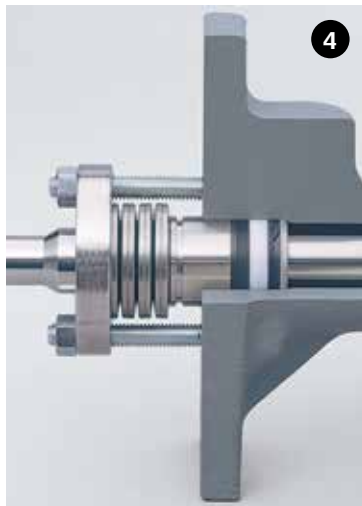
ENVIRO-SEAL® packing, which is available in all Vee-Ball valves, helps meet stringent emission control requirements.
